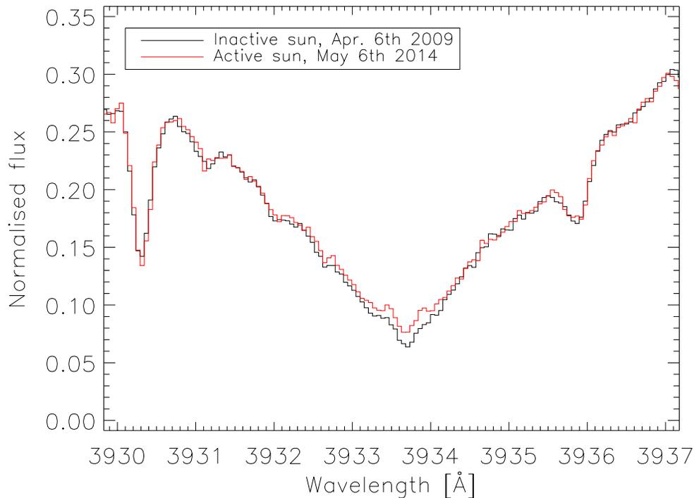
Figure 1: Spectra of TIGRE (formerly Hamburg Robotic Telescope) and its HEROS spectrograph ( $R=20\,000$  resolution) show the solar Ca II K line core at its basal flux level in 2009 ( $S=0.15$ , Schröder et al. (2012)) and at an only moderately active level in 2014 ( $S=0.17$ ). Note that the instrumental profile causes a broadening of about  $0.2\text{ \AA}$ , which levels the computed emission core of Fig. 2 significantly.
