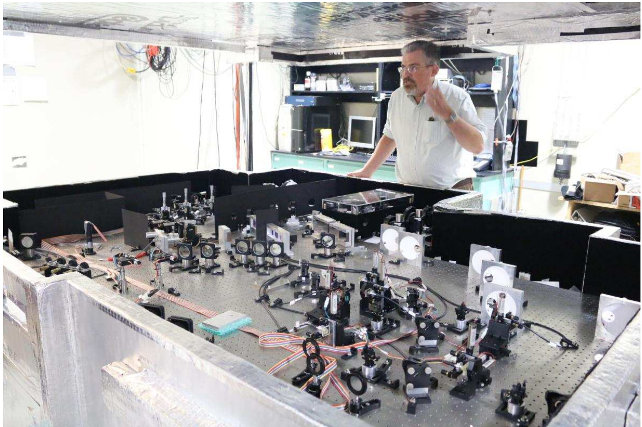
Don Hutter explains the beam combiner of the Navy Precision Optical Interferometer.
