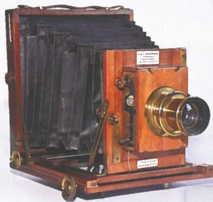
Mary's folding camera that took both dark slide and roll-film attachments. Made by Underwood, Birmingham, c. 1898. Labelled 'The Field', half plate model. Made from mahogany with leather bellows
