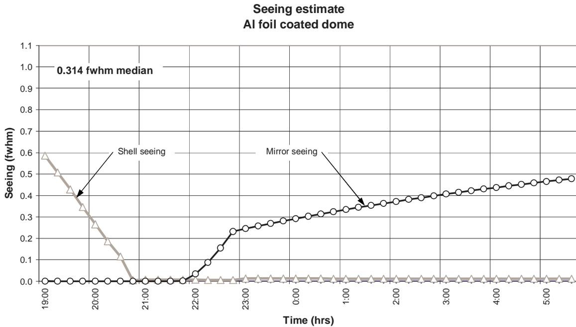
Figure 9. Coating the dome shell with self adhesive aluminum foil tape (3M #425) reduces shell seeing to near zero by 21:00. After 22:00 mirror seeing begins and increases through the remainder of the night.
