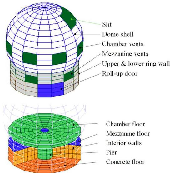
Figure 4. Exterior and interior features of the WinTherm<sup>®</sup> model. The telescope structure was modeled as a single node representing its exposed surface area and thermal capacitance.
