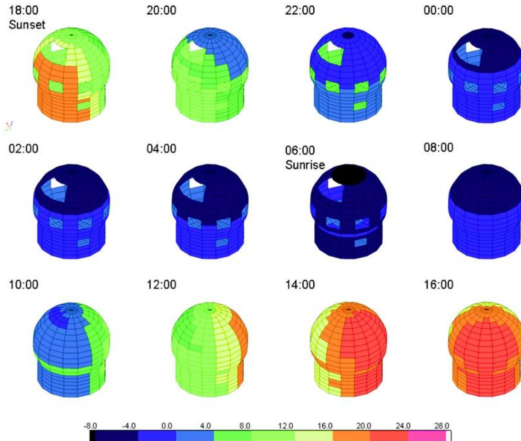
Figure 5. Transient thermal model over a 24 hour period from sunset at 18:00 hours at upper left. Progressive cooling due to radiation to the night sky can be seen from 22:00 to 08:00; the track of the sun can be discerned as it advances over the dome surface from 10:00 to 18:00.
