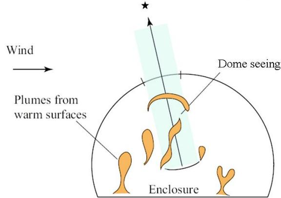
Figure 2. Warm areas of the enclosure including e.g. floor, walls, telescope or other structure generate rising plumes of warm air. As these plumes pass into the optical beam they are observed as dome seeing. Illustration adapted from Dalrymple [2004].
