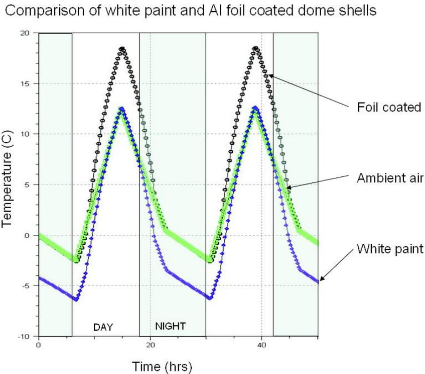
Figure 8. When coated with white paint a dome shell stays closer to ambient air temperature during the day but cools below ambient at night; the aluminum foil-coated shell overheats during the day, but stays closer to ambient temperature at night.
