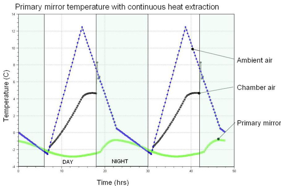
Figure 10. Extracting heat from the primary mirror can reduce its temperature and so reduce mirror seeing. Here a modest but continuous (24-hr) extraction rate of 135 W from the back of the mirror has been modeled.
