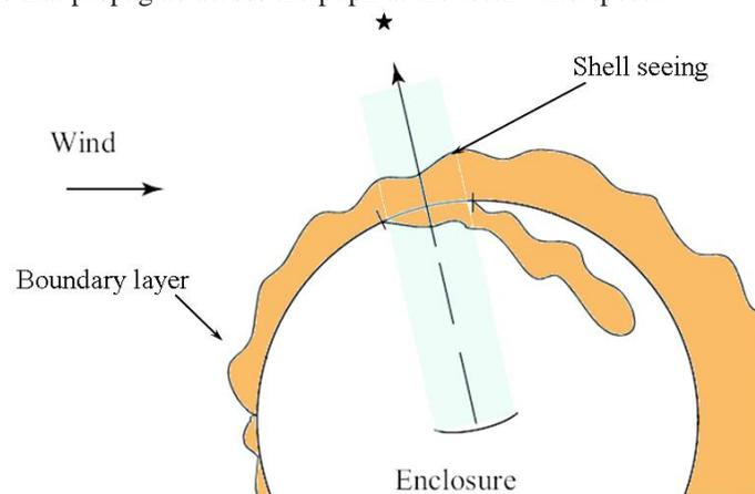
Figure 1. Shell seeing results from air heated or cooled by convection from the shell of the dome. As this air passes over the optical beam it is observed as shell seeing.
