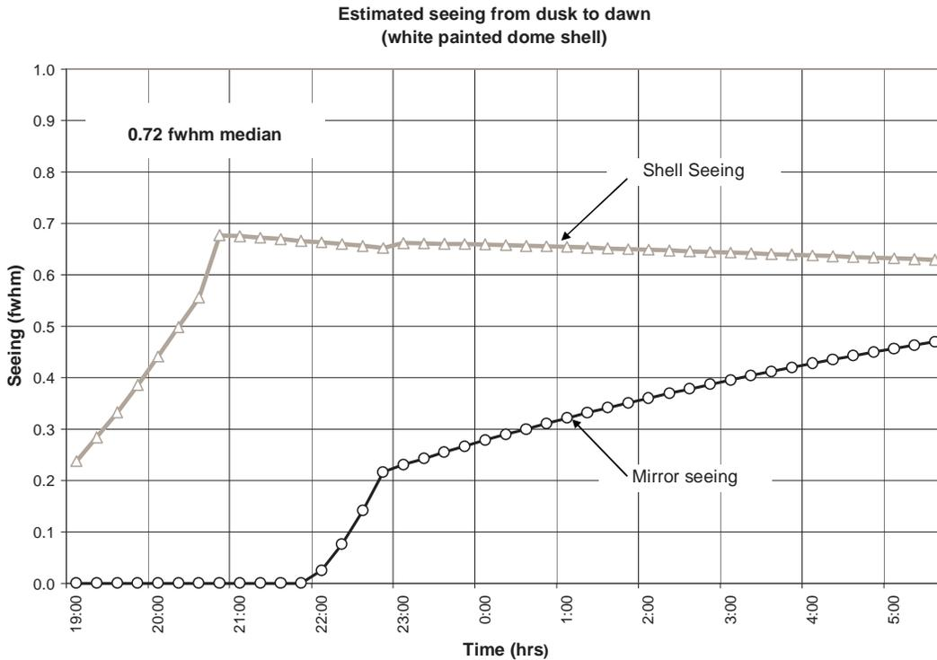
Figure 7. Night time seeing estimates based on the temperature data in Figure 6. The white painted dome shell rapidly cools by radiation to the night sky until it reaches an equilibrium balanced by convection. Consequently shell seeing rapidly increases to a plateau. Mirror seeing starts when the chamber air temperature falls below the primary mirror and increases through the night.
