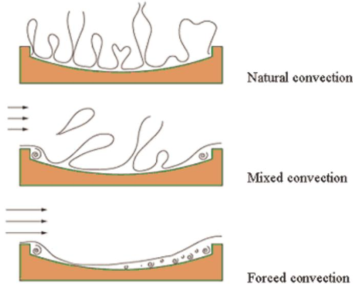
Figure 3. Mirror seeing has three regimes according to the velocity of air moving over the mirror surface. Adapted from Dalrymple [2003]
