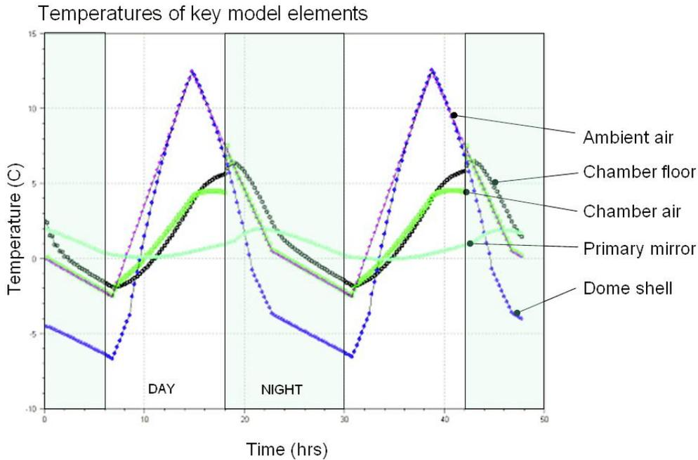
Figure 6. Time history plot of the key elements over a 48 hour period starting at midnight. The white painted dome shell cools about 5C below ambient by radiation to the night sky. The primary mirror temperature lags behind the chamber air temperature due to thermal inertia. These data were used to generate the seeing estimates in Figure 7.
