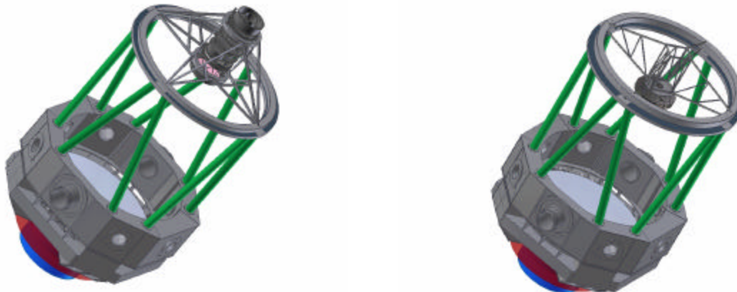
Figure 5-1: Prime Focus Mount Configuration (left); RC Mount Configuration (right)
